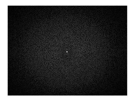
$<sup>^3\,</sup>$  Zero Order: (Power meter reading with DOE / Power meter reading without DOE ) X 100%
